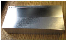
Synchronized point distribution works with your controller's interpolation scheme to provide the smoothest finishes.
